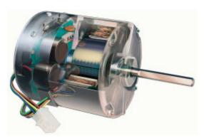
The ECM is a DC motor, with a permanent magnet rotor. Motor windings (electro-magnets) are placed around the rotor. An internal microcontroller sequentially connects DC current to each winding, causing the motor to turn. The timing, duration and firing order of these current pulses controls the motor output and rotational direction.
